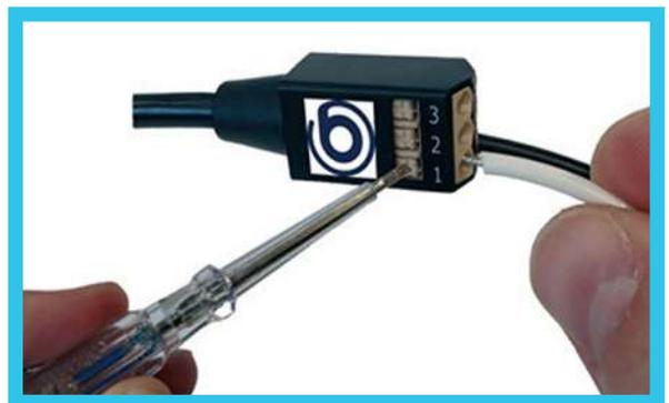
6. Now push the CT secondary leads into the RJ12 adaptor terminals for your phase type as shown on the next page. The white cable of each CT connects to either terminals 1, 2 and 3 of the side showing the Best.Energy logo. The corresponding black cable of each CT connects to terminal of same number on the opposite side of the terminal block.
