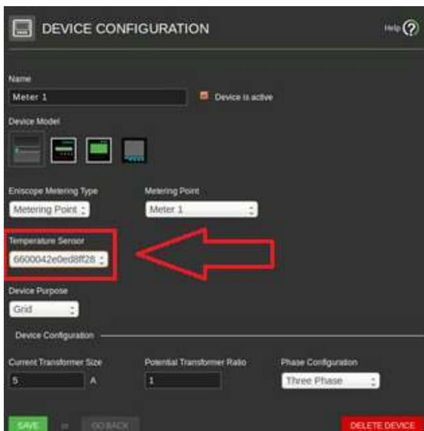
To avoid confusion with multiple sensors, connect the first sensor physically, configure the meter via the software, then add the next sensor physically and repeat. This way as each new probe is added, it will appear as a newly available temperature sensor to add in the metering point. If necessary mark each probe with an identification number so you can find it in the future.
