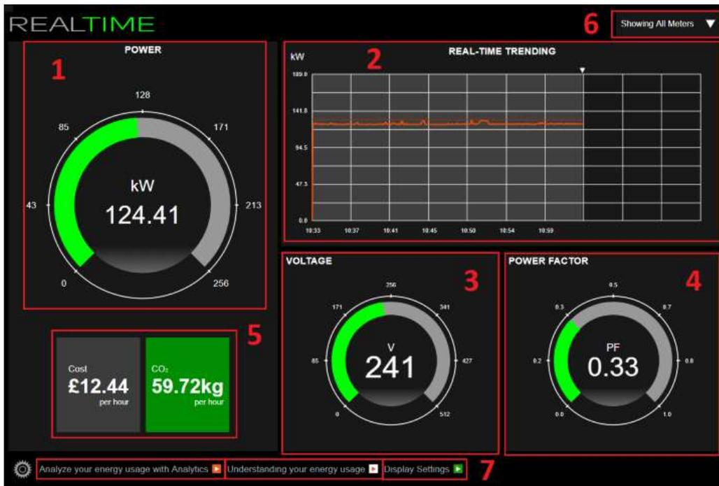
To access the Real time display you can select from the HTML5 or FLASH version at the bottom of the menu, while logged into Enscope. Otherwise type the Enscope IP Address in your web browser address bar, (i.e 192.168.0.127) for direct link to the real time display.
