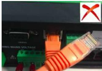
3. Check your computer is on the same IP range, for this you ideally need to check with your IT expert. As depending on the size of your network and setup, you could be using multiple switches and IP ranges. If in doubt trace the cable from the Eniscope to the nearest hub and connect your computer to the same hub via cable.
