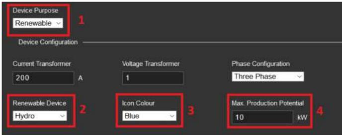
1. The first step is to set up your Renewable device information in 'Setup Your Devices' in addition to the normal settings explained under 'Meter setup' section.
