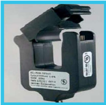
3. Attach the current transformer around the conductor to be monitored without placing excessive strain or pressure. Do not route the leads over sharp edges and take care to fit the CT with the arrow in direction of flow/load.
