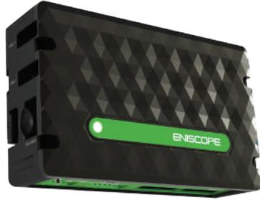
2. Check the Eniscope is connected to your network, you should see a Green LED on the Ethernet socket after powered on. If not check your cable for signs of damage or check the retaining clips on the plugs are not damaged or try another cable.
