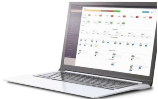
From this website you can setup remote scheduling for your aircon systems, such as ensuring they off outside of operating hours or scheduling multiple units to be all on at peak day heat, while operating just 1 aircon for the evening or overnight conditions.
