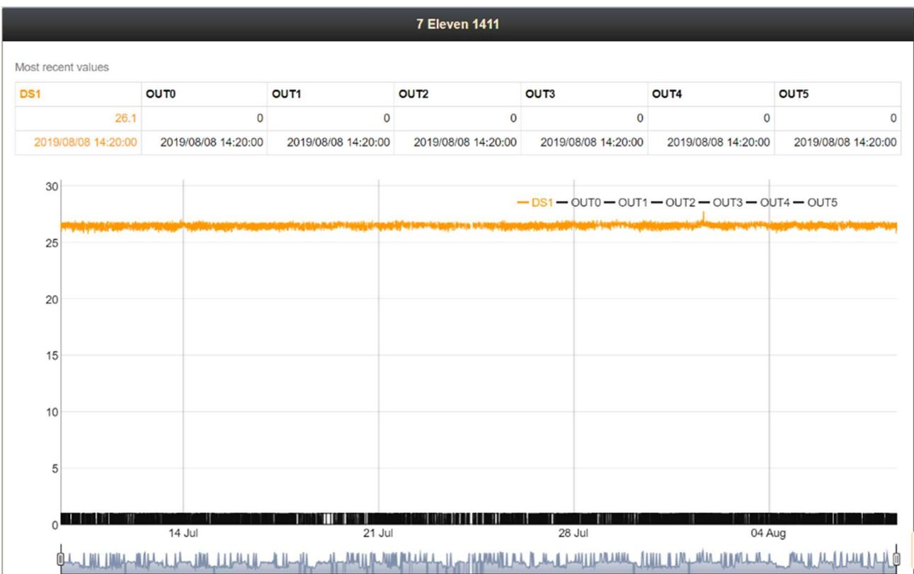
Selecting the chart option, you can see data for the last month for the ACES2 temperature sensor, if setup correctly you should see a reasonable controlled tight formation like the above example. If your temperature varies to much, you can scroll to a specific time or day with the sliders at the bottom of the graph to analyse.
